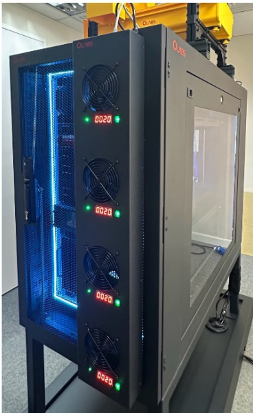
Smart Fan Unit – Slave (OIF-F4S-1) Front door 4 fans – intake airflow
