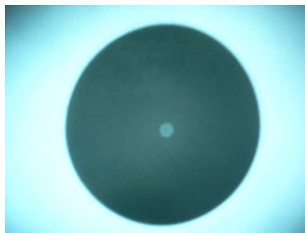
Diagram-2: Clean and defect free end-face inspection under 400x microscope
